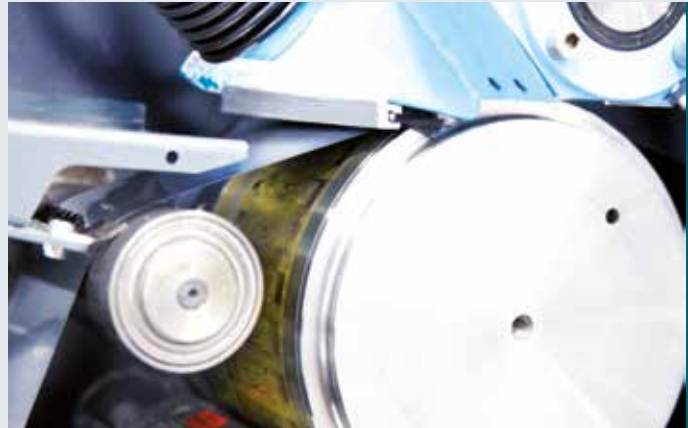
MAGNETIC CYLINDER • with exchangeable cliché
