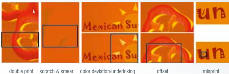
double print scratch & smear color deviation/underinking offset misprint
