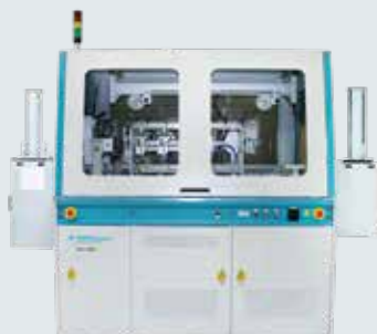
SCI 5001 Fully-Automatic Implanting of IC Modules into Plastic Cards
