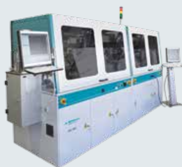
DICL 5000 Fully-Automatic Cavity Milling and Implanting of Modules for Dual Interface Cards
