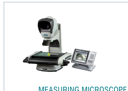
MEASURING MICROSCOPE Measuring of embossing distances
